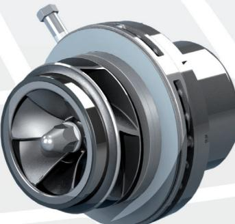
Closed impeller statically and dynamically balanced. The axial thrusts are balanced by back vanes, for the best axial balancing independently from suction pressure.
