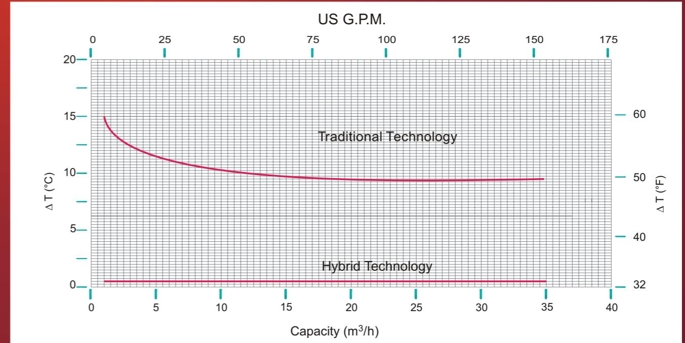
Hybrid technology reduces greatly heat generation in the rear casing region. This benefit is particularly important when pumping low boiling liquids.
