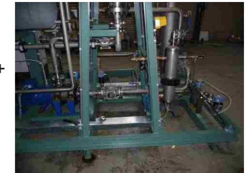
SC MAG-M65 / 5 stages, for pumping of ISOBUTYLENE Q=35 mc/h, H= 40m; Ningbo - China.
