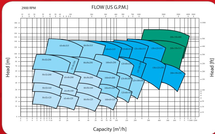
CN SEAL-M Design Metallic mechanically sealed single stage centrifugal pump. Dimensions and delivery data to ISO/EN 2858/5199 Frame-mounted. ATEX 94/9/EG.
